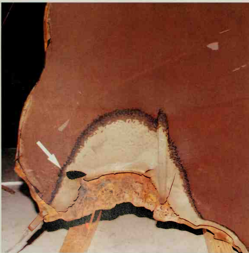
At upper left is the aft segment burn viewed from inside the casing; the lower photo is a closeup of the same section. The latter photo shows a hole (arrow) where the flame plume may have burned through the casing from the outside. At right is a composite view of the burn above and below the aft field joint.
